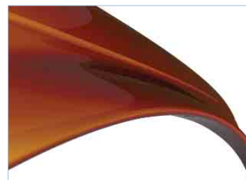
Figure 2. Then use a new feature in Alias Studio Tools 11 to add a tubular flange to the hole.
