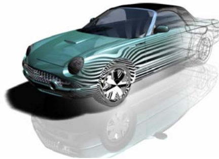
Object with Class A-surfaces and Highlight Diagnosis Display
