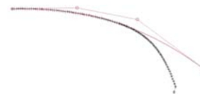
Sectional point data and Bezier curve
